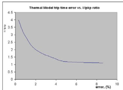
The graph shows the trip time error with respect to the ratio of cable load and thermal model pickup setting. With a smaller I/lpk ratio, the time error tends to be higher, as accumulated through the logarithmic formula, the measurement error, and the time of measurement. For higher I/lpk ratios, the time to trip is substantially more accurate. Each point on the graph represents a trip time error, with the I/lpk ratio kept constant during the test.
