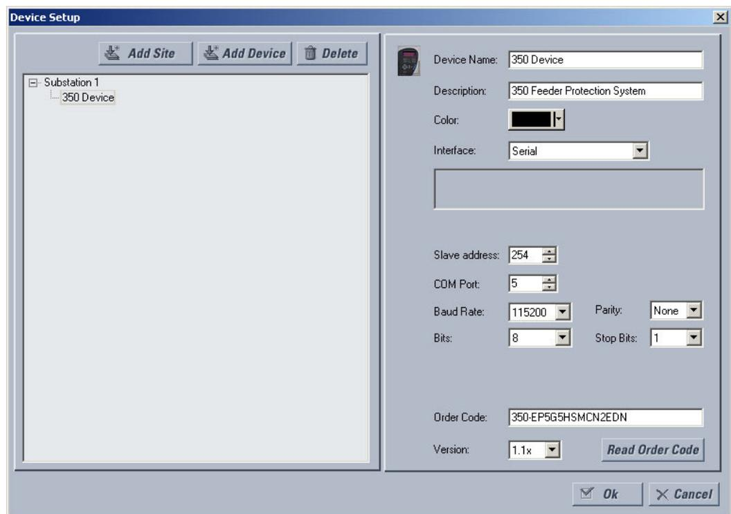
8. Click the **Read Order Code** button to connect to the 350 device and upload the order code.
