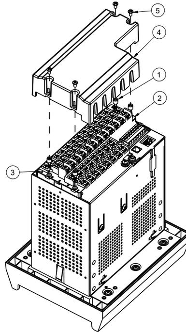
1. Place 4 custom standoffs (item#1) using the suggested tightening torque of 8lb-in in the following order:
