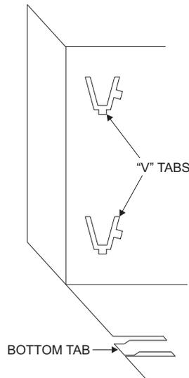
1. From the front of the panel, slide the empty case into the cutout until the bottom tab clicks into place (see above).
