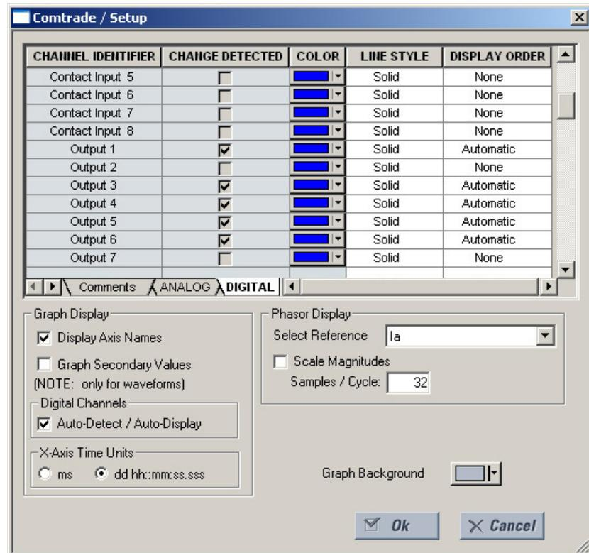
Change the color of each graph as desired, and select other options as required, by checking the appropriate boxes. Click **OK** to store these graph attributes, and to close the window. The Waveform Capture window will reappear based on the selected graph attributes.
