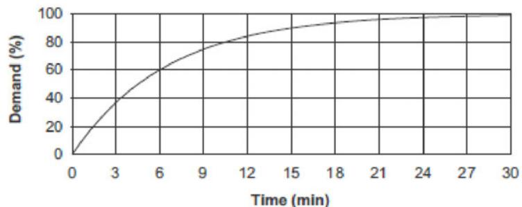
The 90% thermal response time characteristic defaults to 15 minutes. A setpoint establishes the time to reach 90% of a steady-state value, just as with the response time of an analog instrument. A steady-state value applied for twice the response time will indicate 99% of the value.
