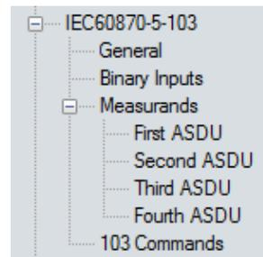
**PATH:** SETPOINTS > S1 RELAY SETUP > COMMUNICATIONS > IEC61870-5-103
