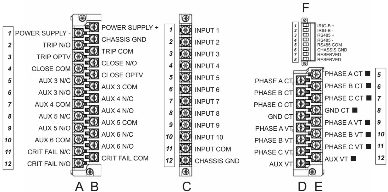
Figure 2-33: 350 Terminal Identification - Non-drawout
