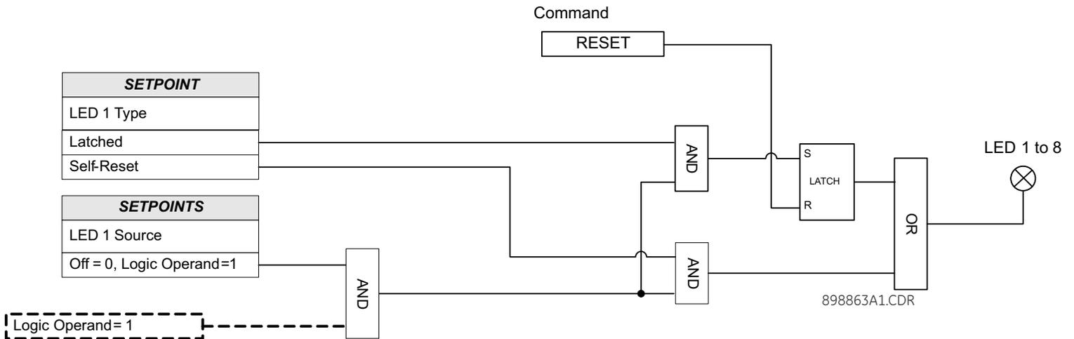
When the LED TYPE is Latched, the LED stays lit even after the value of the operand (flag) selected as a trigger drops down (resets). The LED can be turned off by either pressing the RESET pushbutton, or by executing a reset command via communications. When the LED TYPE is Self-reset, the LED resets after the logic operand value drops down (resets).
