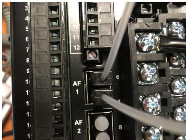
**Installing the loop sensor fiber with a sensor fiber extension:**
