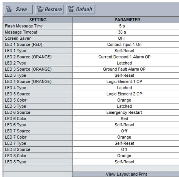
6. In the **Setpoint > S1 Relay Setup > Front Panel** dialog box, click **Save** to save the values into the 350 . Click **YES** to accept any changes. Click **Restore** to retain previous values. Click **Default** to restore Default values (all LEDs Off and colors Orange).
