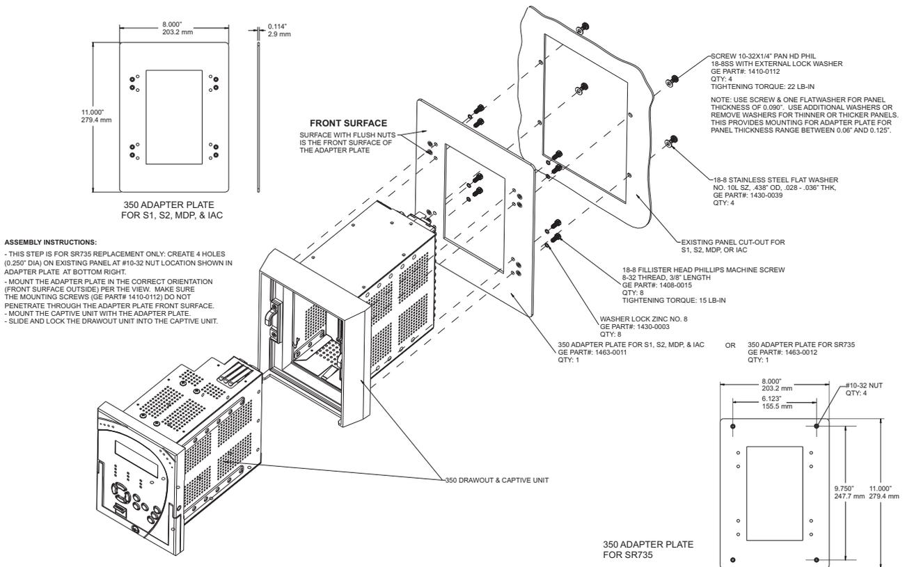
Figure 2-10: Non-drawout - Adapter plate mounting
