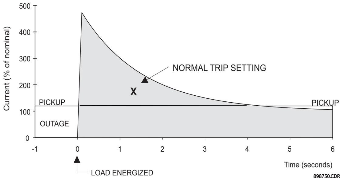
The relay detects Cold Load condition (Cold Load Pickup armed), if the currents on all three phases drop below 3% of the CT nominal rating for the period of time greater, than the Outage Time Before Cold Load setting. The Cold Load condition can be immediately initiated (Outage Time Before Cold Load timer bypassed), by asserting a contact input selected for External CLP Initiate.
