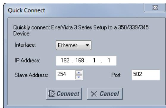
As indicated by the window, the "Quick Connect" feature can quickly connect the EnerVista 3 Series Setup software to a 350 front port if the USB is selected in the interface drop-down list. Select "SR3 Relay" and press the **Connect** button. Ethernet can also be used as the interface for Quick Connect as shown above.
