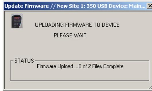
6. The EnerVista 3 Series Setup software will notify the user when the 350 has finished loading the file. Carefully read any displayed messages and click **OK** to return the main screen. **Cycling power to the relay is recommended after a firmware upgrade.**
