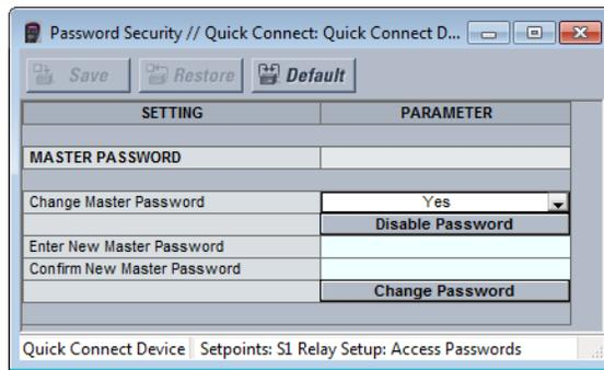
2. Now that the Master Password has been programmed, enter it again to log in to the Master Access level. The Master Level permits setup of the Remote and Local Passwords. If the Master Password has been lost, contact the factory.
