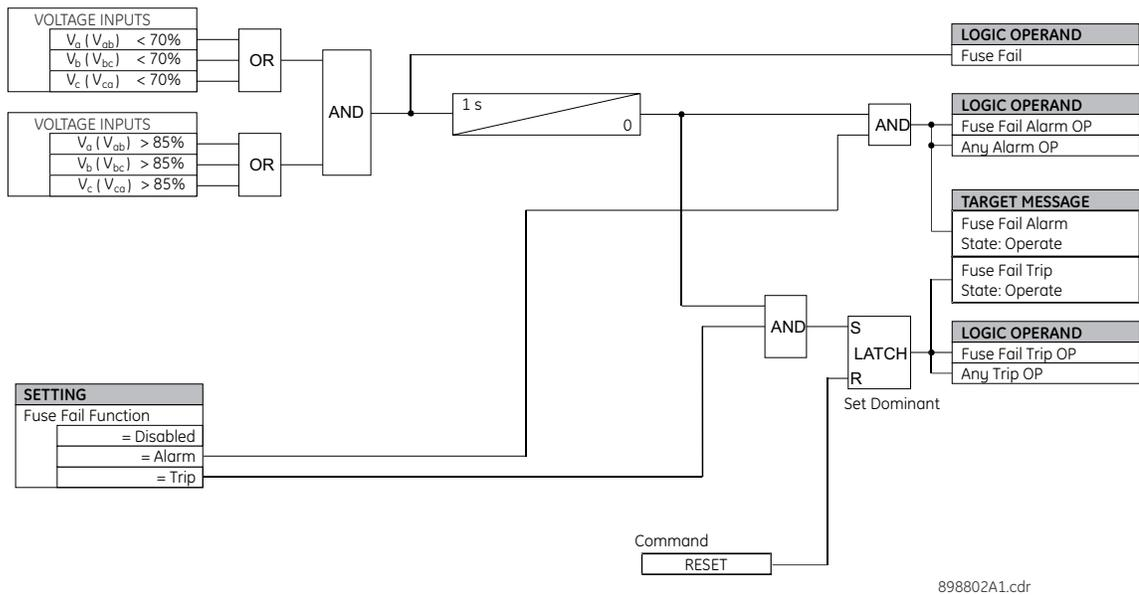
NOTE: The VTFF uses phase to neutral voltages  $V_a$ ,  $V_b$  and  $V_c$  when "Wye" VT type is selected under Voltage Sensing/VT connections setpoint, and uses phase-phase voltages  $V_{ab}$ ,  $V_{bc}$  and  $V_{ca}$  when "Delta" type is selected comparators.
