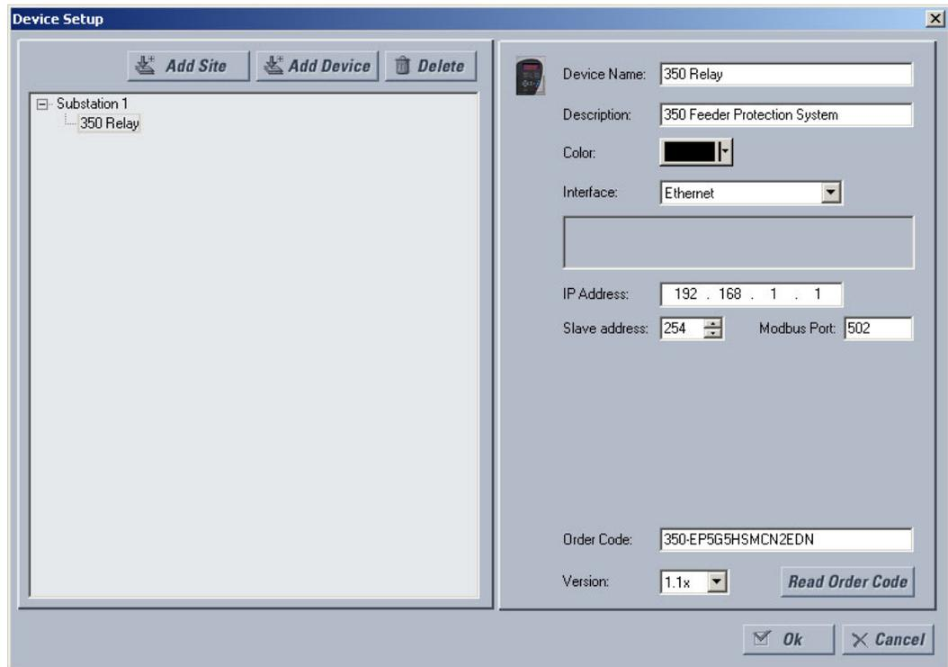
8. Enter the IP address, slave address, and Modbus port values assigned to the 350 relay (from the S1 RELAY SETUP > COMMUNICATIONS > ETHERNET menu).
