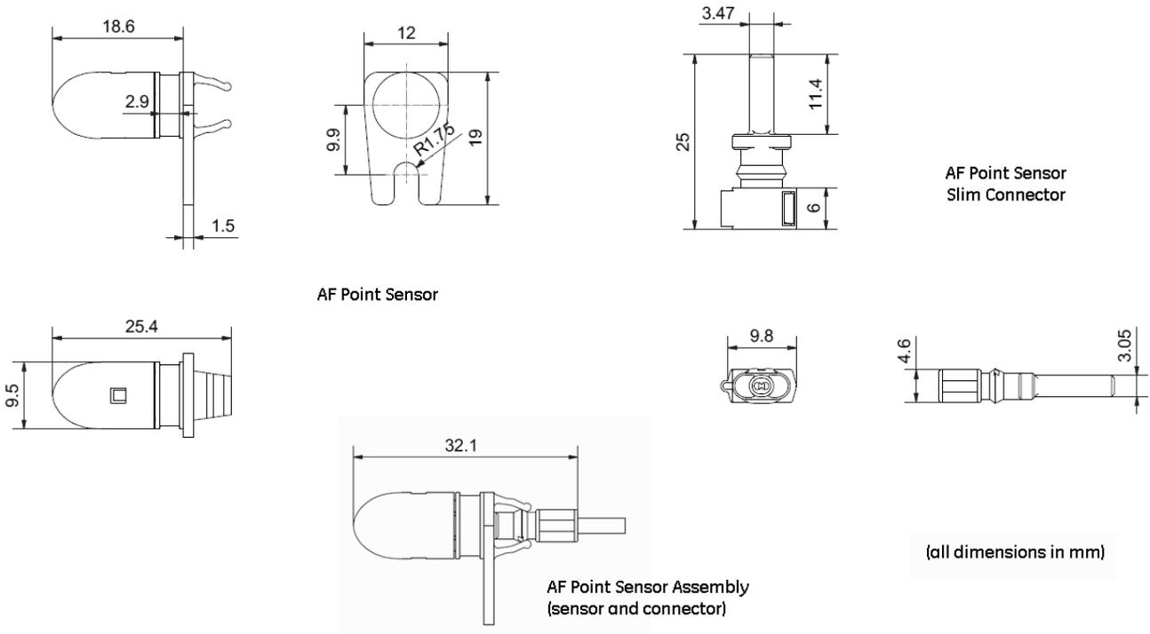
Figure 2-17: Duplex connector dimensions (point sensor, and sensor fiber extension for loop sensor)
