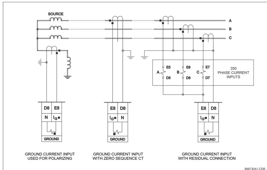
The polarizing signal for the Ground Directional element is based on the zero sequence voltage. Depending on the relay's order code, the zero sequence voltage used for the polarizing voltage, is either calculated, when three-phase voltages are available, or is measured from the auxiliary voltage input  $V_x$  when the three-phase voltages are not available. For those relays with available phase VTs, the polarizing voltage for the Neutral directional element is calculated as follows:
