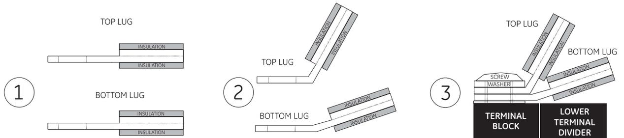
Figure 2-30: CORRECT INSTALLATION METHOD
