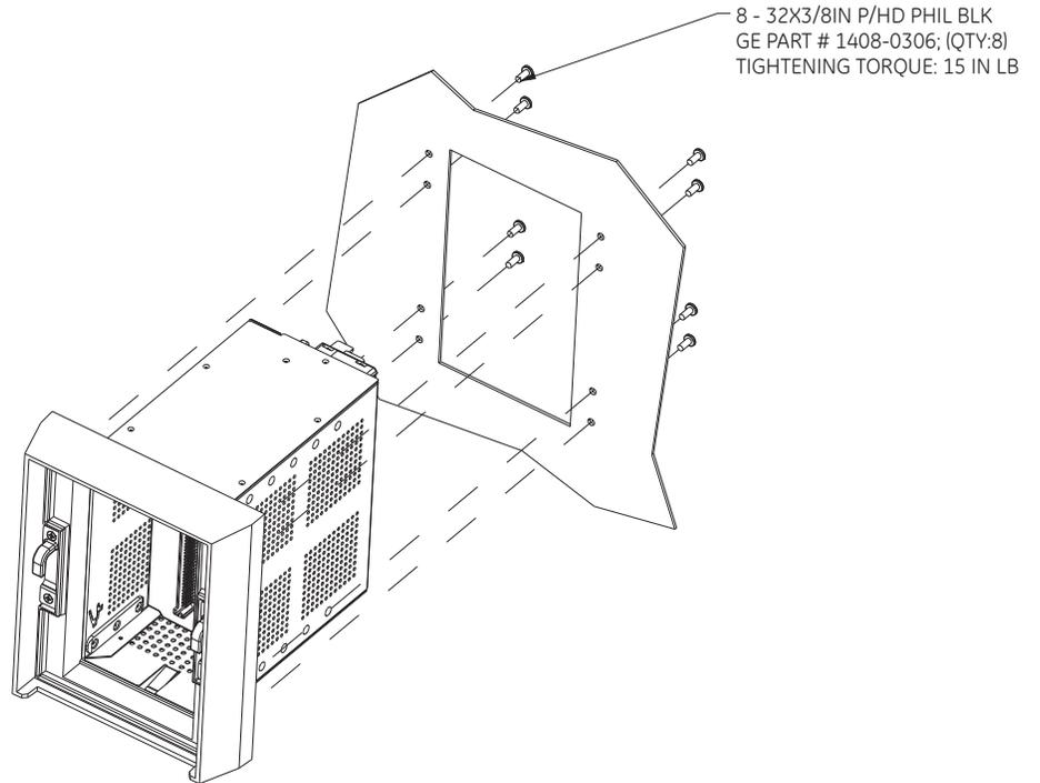
Figure 2-5: Standard Panel mounting - Non-drawout
