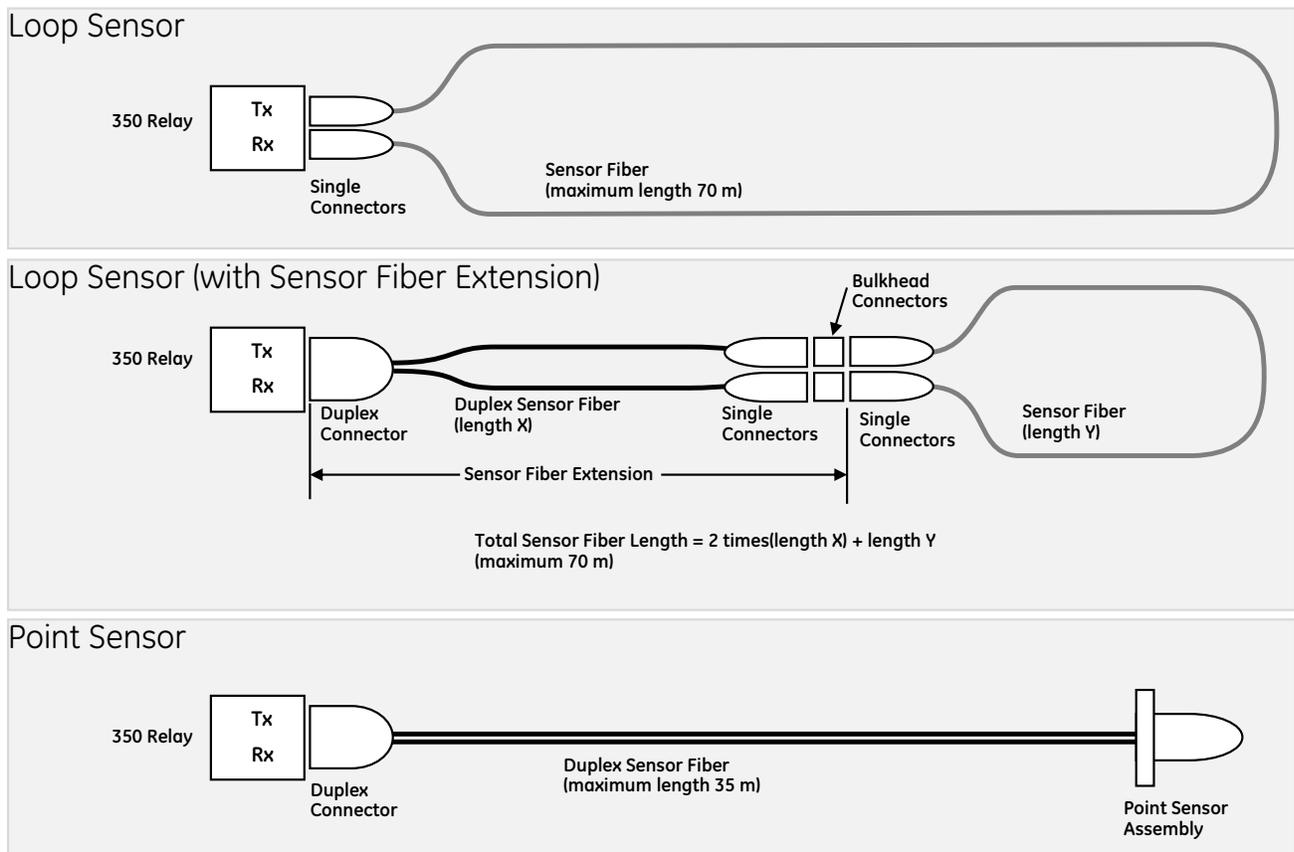
Arc flash sensors of either type can be connected to any of the four arc flash ports on the back of the 350 relay, as shown.
