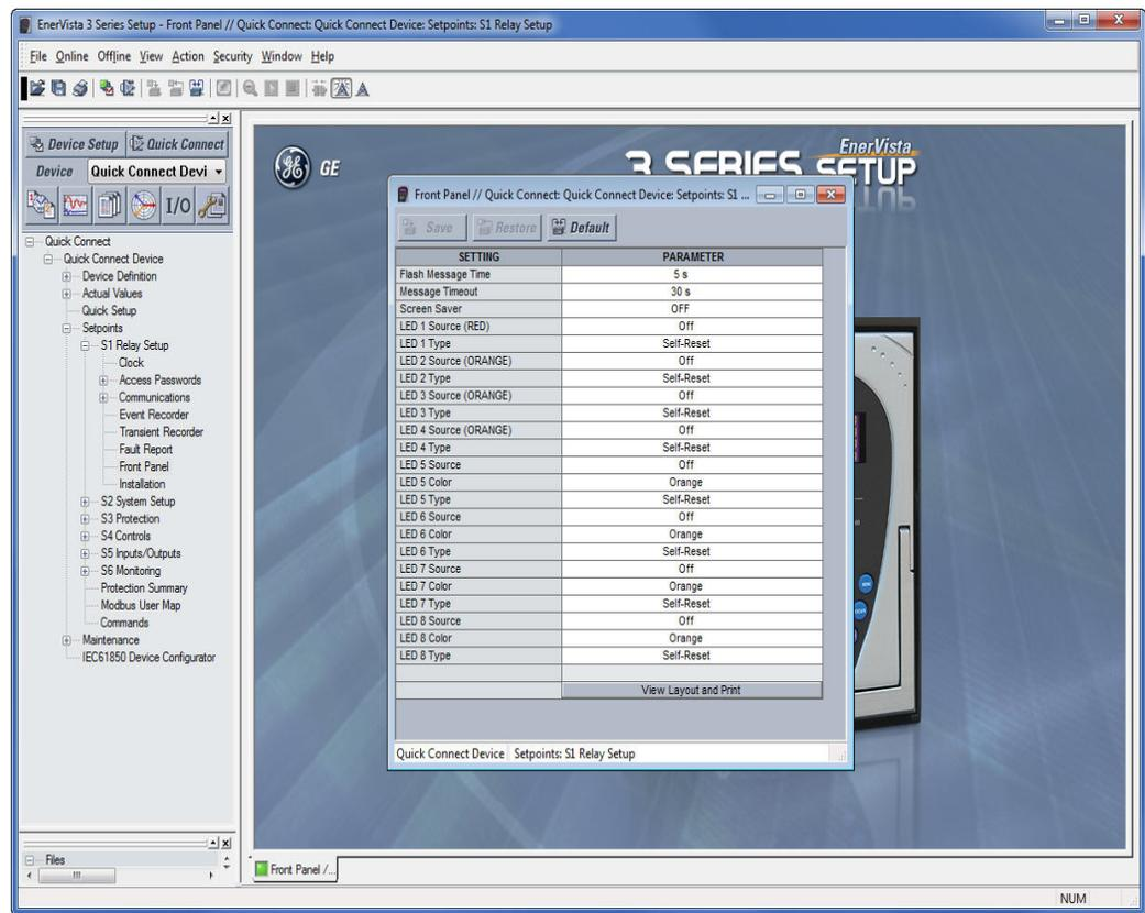
The 350 Site Device has now been configured via the Quick Connect feature for either USB or Ethernet communications. Proceed to *Connecting to the Relay* below, to begin communications.
