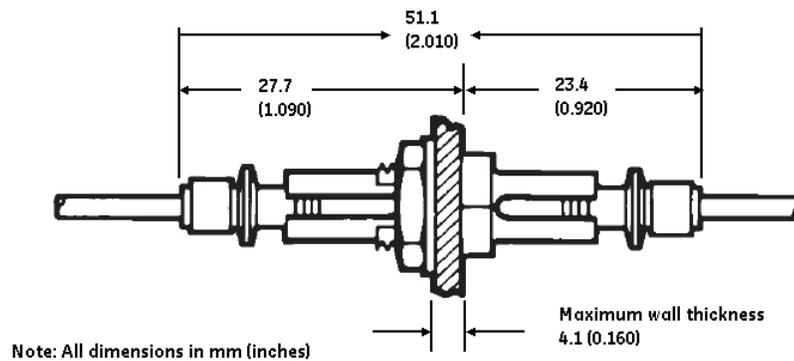
Before installing the AF sensor units, ensure that all other drilling and installation is complete to minimize possible damage to the sensitive unit and connected sensor fiber cable.
